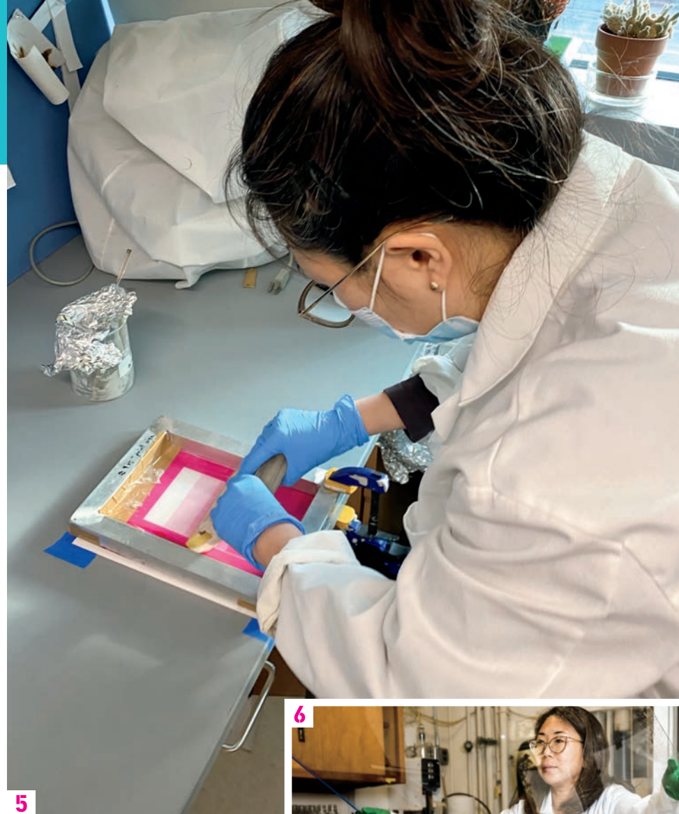
5. Squeezing the E. coli ink across a screen to create a test print. The ink goes on clear; 6. Kim covers a tray with prints in water for an experiment using different carbon sources in the ink; 7. Pouring more water into prints in the incubator; 8-9. Incubated test prints depicting birds.
